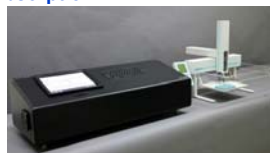
Figure 1. Laboratory \delta^2\text{H} and \delta^{18}\text{O} measurements using the custom LGR LWIA. 240 complete unknown sample measurements recorded in 43 hours with a precision of \pm 0.30 ‰ in \delta^2\text{H} and \pm 0.058 ‰ in \delta^{18}\text{O} . The average values ( -78.92 ‰ for \delta^2\text{H} and -11.53 ‰ for \delta^{18}\text{O} ) agree with the actual values ( -79.0 ‰ for \delta^2\text{H} and -11.54 ‰ for \delta^{18}\text{O} ) to within the instrumental precision.
